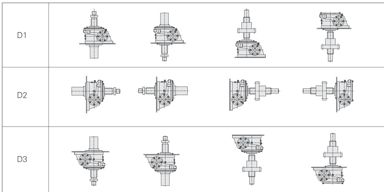
Note: When applying D3 mounting position, performance level of foot-mounting bolts should be above 10.9.
