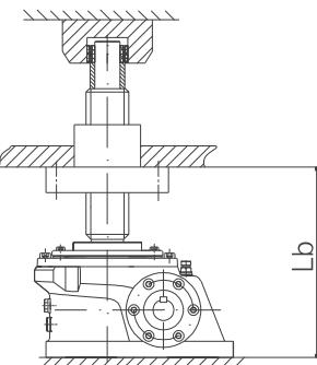
Calculation example: J200NU-1200HA-D1 Input speed is 1200r/min, run under shaft end support, check according to outline dimension and transmission capacity:
