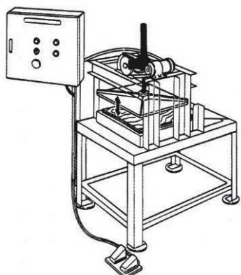
Height adjustment of straightening machine
