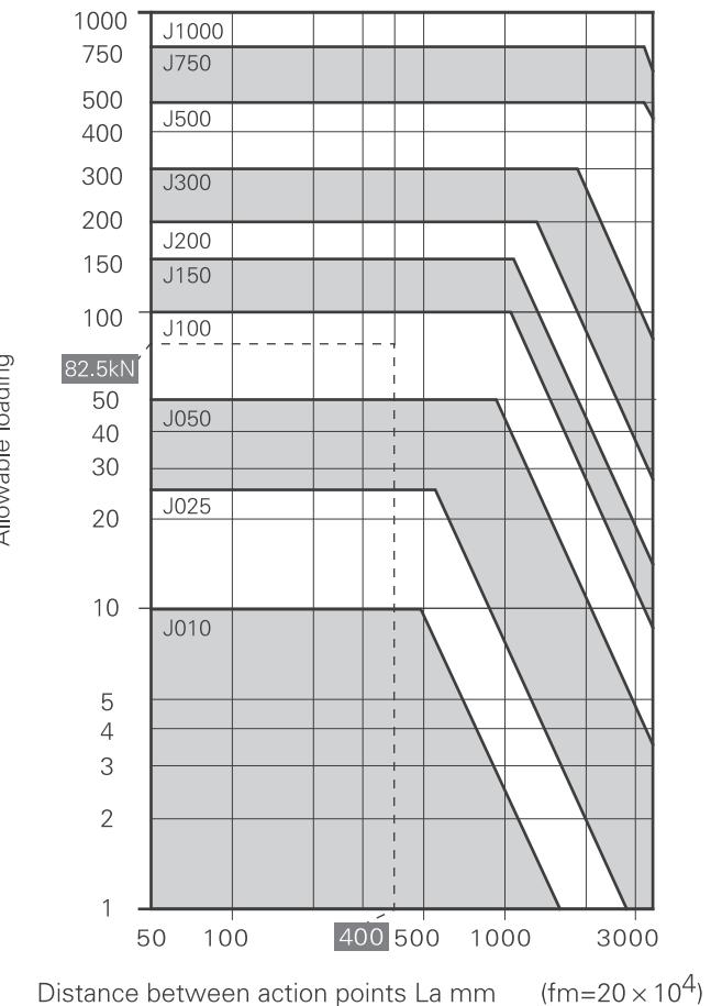
“—” means loading W=82.5kN, ( safety coefficient SF=4 ) point distance La=400mm ( foundation fixed shaft end supporting fixing fm=20 × 10<sup>4</sup> ) as an example; at this time, you can select ladder screw elevator J100 which can satisfy crossing point of vertical and horizontal axis.
