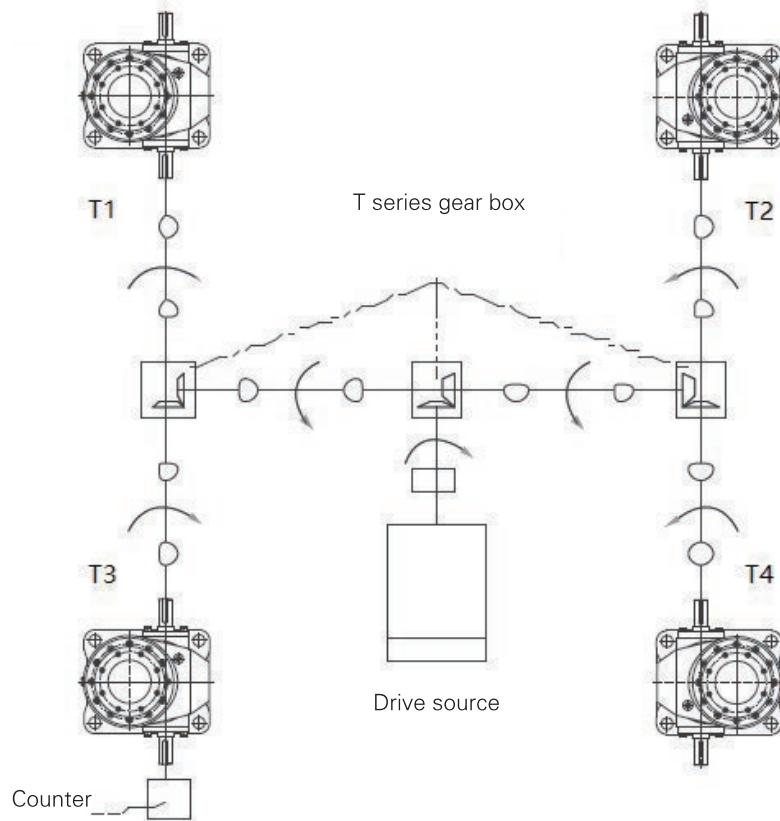
2. Determine the required drive unit capacity Pt with input n and overall  $T_t$  determined in 1.
